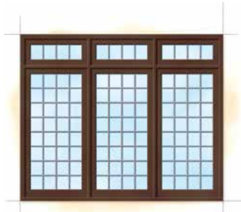
Casement and transom window combination (exterior)
